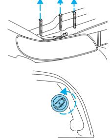
5. Disconnect the electrical connector from the bulb socket.
